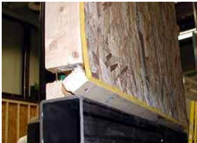
American Plywood Association Shear Wall Test with Cross Grain Bending Failure
