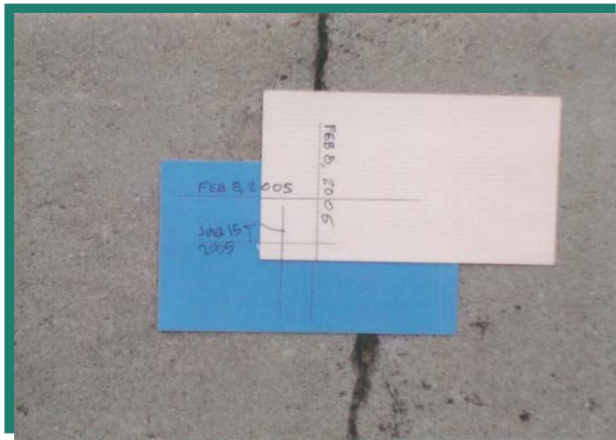
Figure 1: Business Card Crack Monitor. Adhere the cards to the surface, one each side of the crack.
