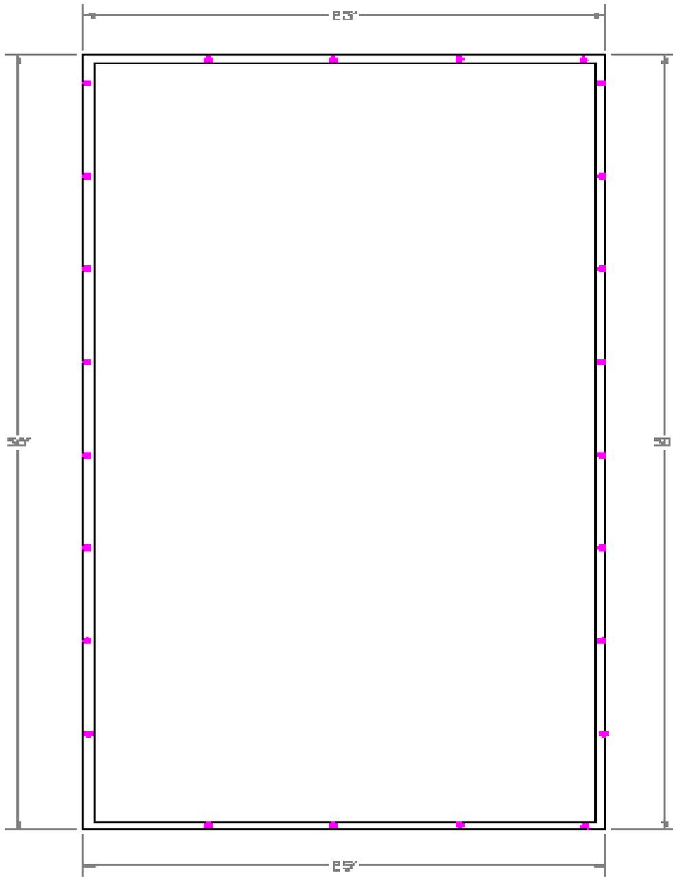
The pink dots represent bolts. If a rectangular house is bolted every six feet, there will be twice as many bolts on the long walls as on the short walls. This means this house is twice as earthquake resistant on the long walls as on the short walls and the failure point will be on the short walls.
