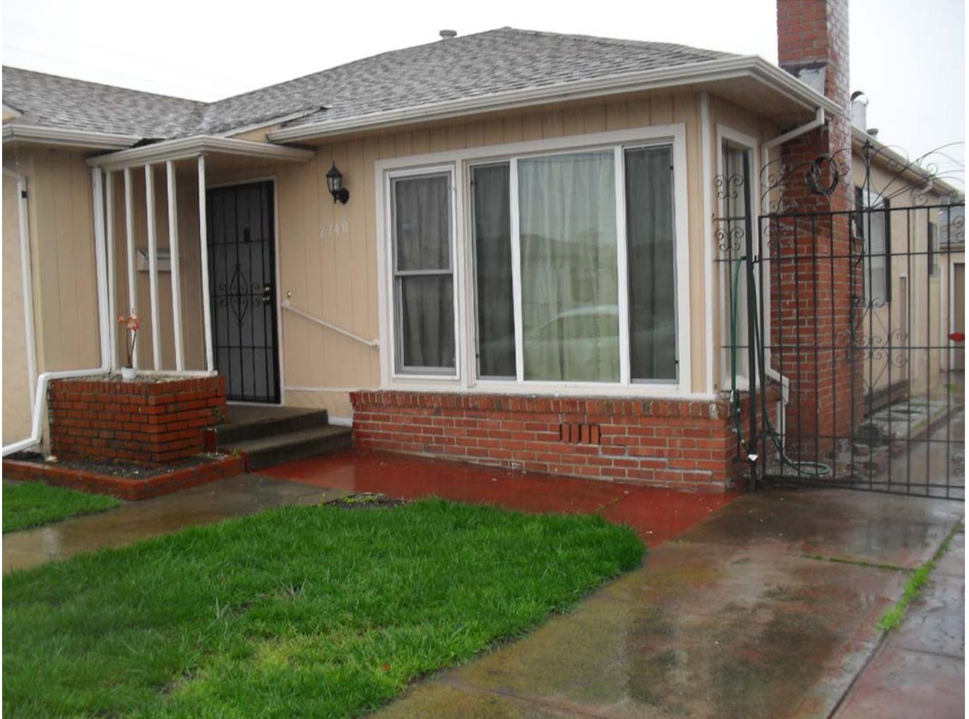
This is a typical newer house built on a level lot. It does not have cripple walls. Bolting was not required by the building code until 1958. If this house was built after this date, we know it was bolted with a ½ inch bolt placed every six feet on the perimeter foundation. However, even though it is bolted according to the code, it can still have structural weaknesses.
