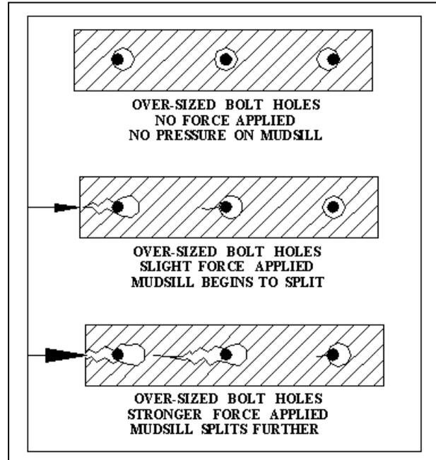
Oversized bolt holes will cause the house to slide on the foundation, at most a few inches, but will not cause a house to slide completely off the foundation.
