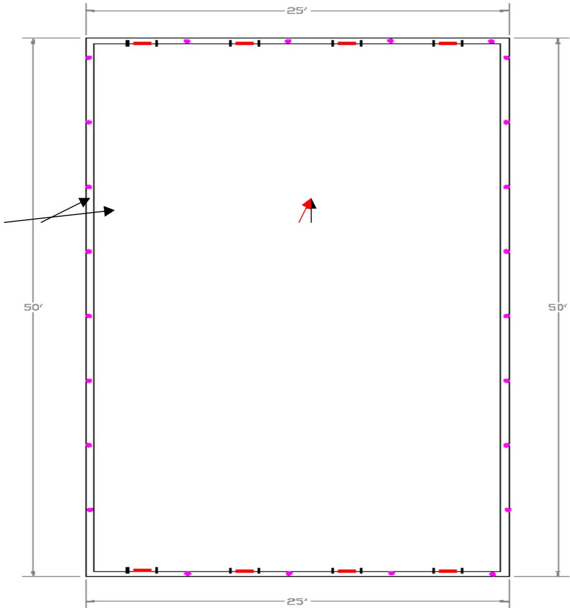
The red lines represent something called foundation anchors, which do the same thing as bolts. After adding these anchors, the bolting strength is now the same on each wall. The two short sides (top and bottom) of the house are now twice as strong as they had been and the earthquake resistance of this house has been doubled.
