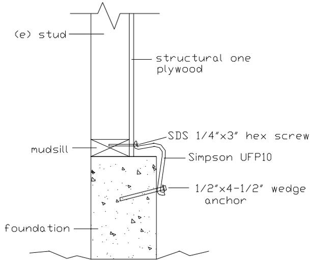
The only thing that needs to be a concern in this method is the fact that the 1/4 by 3" lag screws will only penetrate the mudsill 2 1/2 inches because the plywood takes up 1/2 of an inch. This means that the bolting strength has been reduced by 16%.
