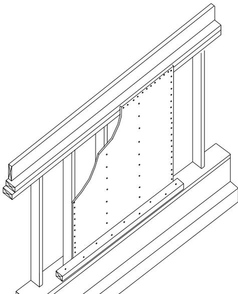
The diagram to the left shows a shear wall made with reverse blocking. The reverse blocking method is quite effective in homes that have wide mudsills. The 2 by 4 reverse-block is nailed to the plywood before the plywood and 2 by 4 are installed on the cripple wall and mudsill.
