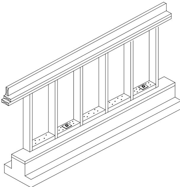
2 x 4 blocks are placed between the upright 2 by 4's and nailed onto the mudsill
